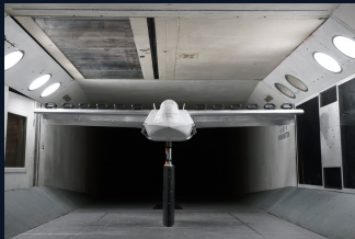
Upper Surface Blown Wing & Adaptive FPS® thrusters – validated thoroughly in the wind tunnel
